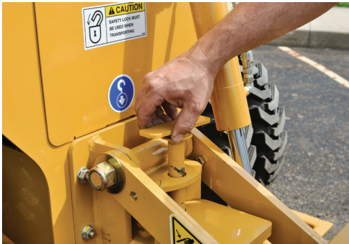
The stump cutter is held to the trailer with simple and secure pins, eliminating chains and binders.
