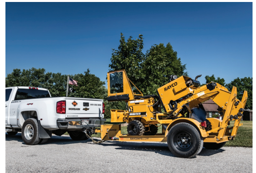
The TRG trailer is equipped with TorFlex suspension and electric brakes.
