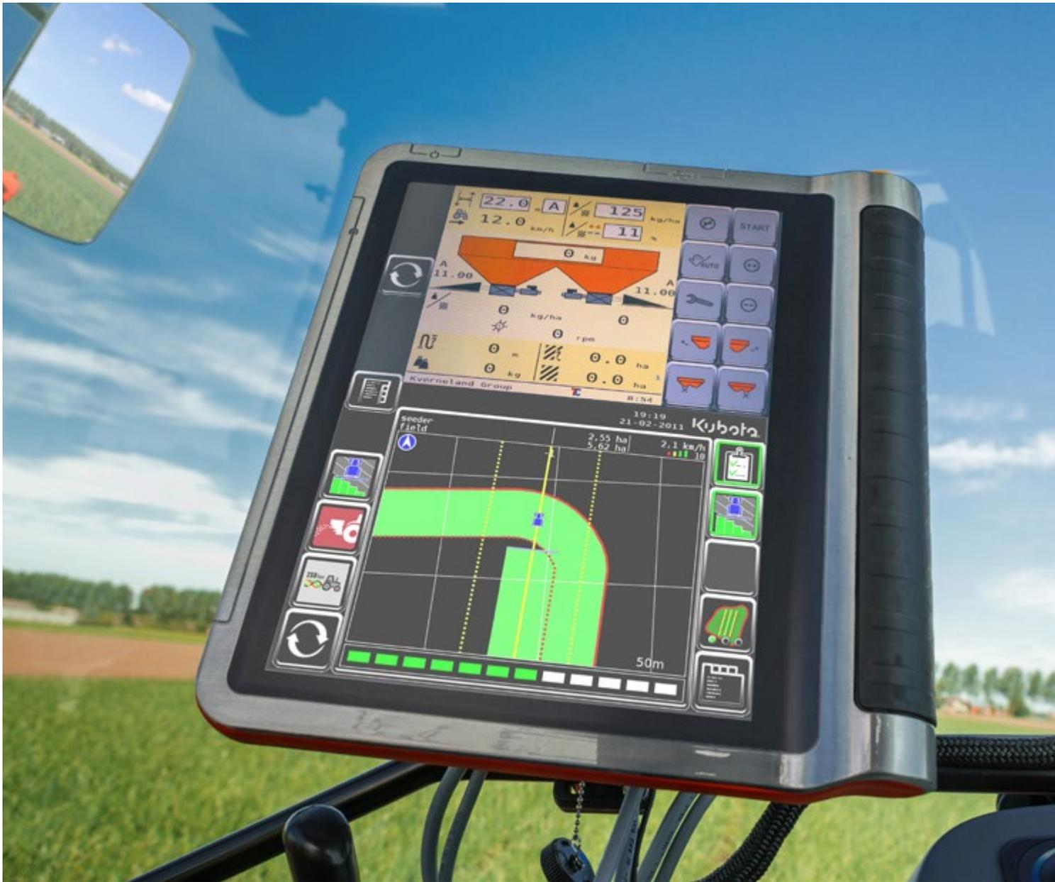
Increase your work efficiency to a new level and make your M5001N an ISOBUS tractor with retrofit kits. This then allows you to fully use any ISOBUS equipment available on the market.
