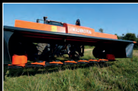
Easy access to the cutterbar with foldable front and side guards.
