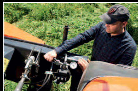
Hydraulic setting of ground pressure.
