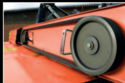
By switching driveline pulleys changing from standard PTO speed of 1000 rpm to 750 rpm is possible.
