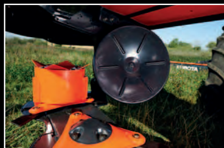
The machine is standard equipped with two swath discs, allowing a swath width of 2.2-2.4m.
