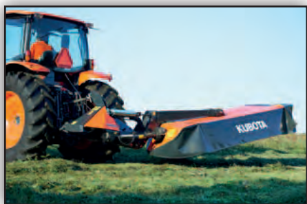
Lifting on headlands via hydraulic cylinder – ample ground clearance.
