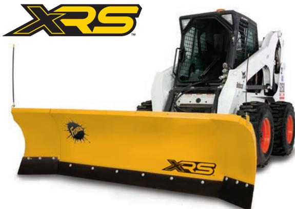
Now you can maneuver snow like never before with the responsive XRS skid-steer plow. Designed specifically for skid-steer applications, this rugged snow fighter automatically retracts the inside wing when full angled and then returns to the scoop position once straight. Blazing efficiency, minus the guess work.
