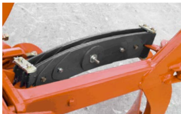
Montage double-pack : 14 lames (1400kg)
