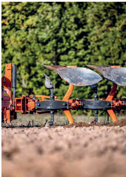
Aero-profile legs to avoid blockages in large residues
