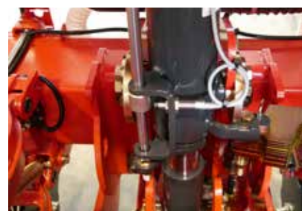
An intelligent two piece hydr. cylinder for best ground following.
