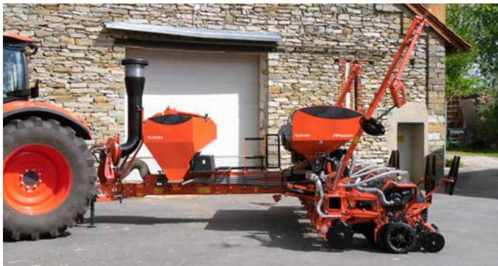
PP1601TF with SX rows and central seed hopper of 870l.
