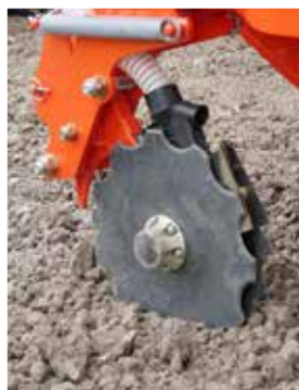
The fertilizer coulter are equipped with maintenance-free roller bearings.
