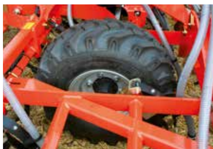
Adjustment of the central wheel by spacer
