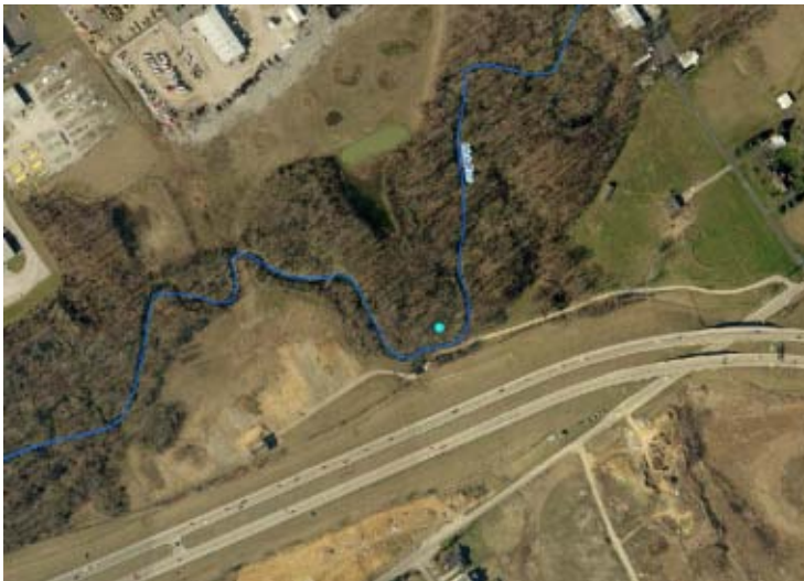
Figure 6-4 Lick Run FEH - Sharp Meander Bend near I-65 Embankment
