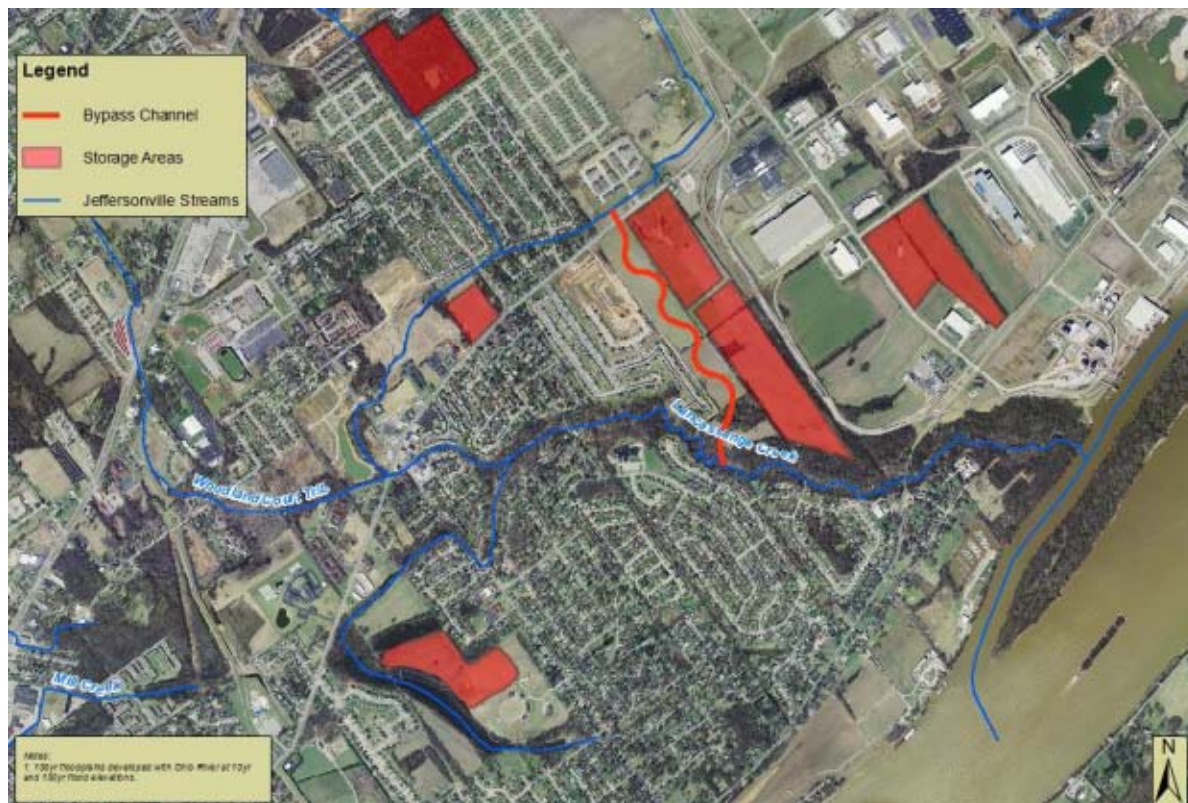
Figure 6-37 Bypass Channel and Storage Basin Layout
