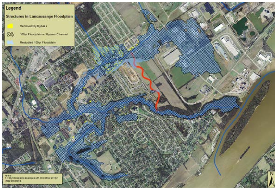
Figure 6-34 Impact of Bypass Channel
