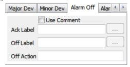
**Ack Label** This is used to write the string displayed when an alarm is acknowledged.
