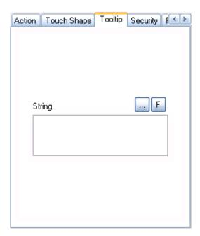
String This is used to enter the string displayed when the mouse is on a corresponding object.
