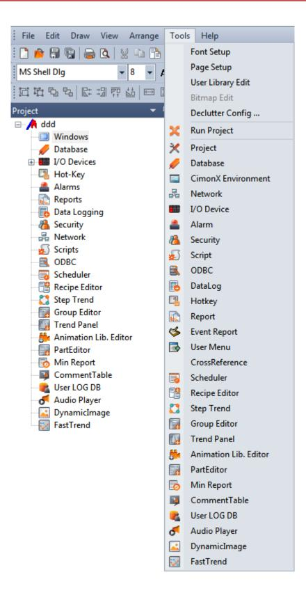
**Font Setup** This is used to assign Font, Style and Size on a page window.
