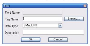
This is used to set up the tag linked with the run result of a SQL or the contents of a statement.
