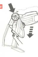
LIFT ADJUSTER HANDLE AND SLIDE SECOND-ROW SEAT FORWARD, ALIGNING ARROWS
