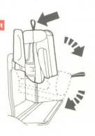
PULL RELEASE STRAP AT REAR OF SEAT, TUMBLE SEAT INTO BIN
