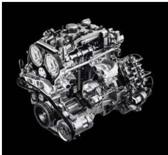
4C's all aluminum 1,750 Turbo Engine with direct-injection.
