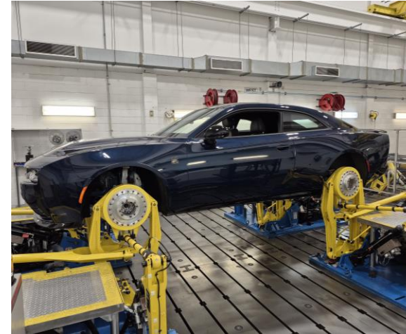
4 DOF Passenger Car Rig
