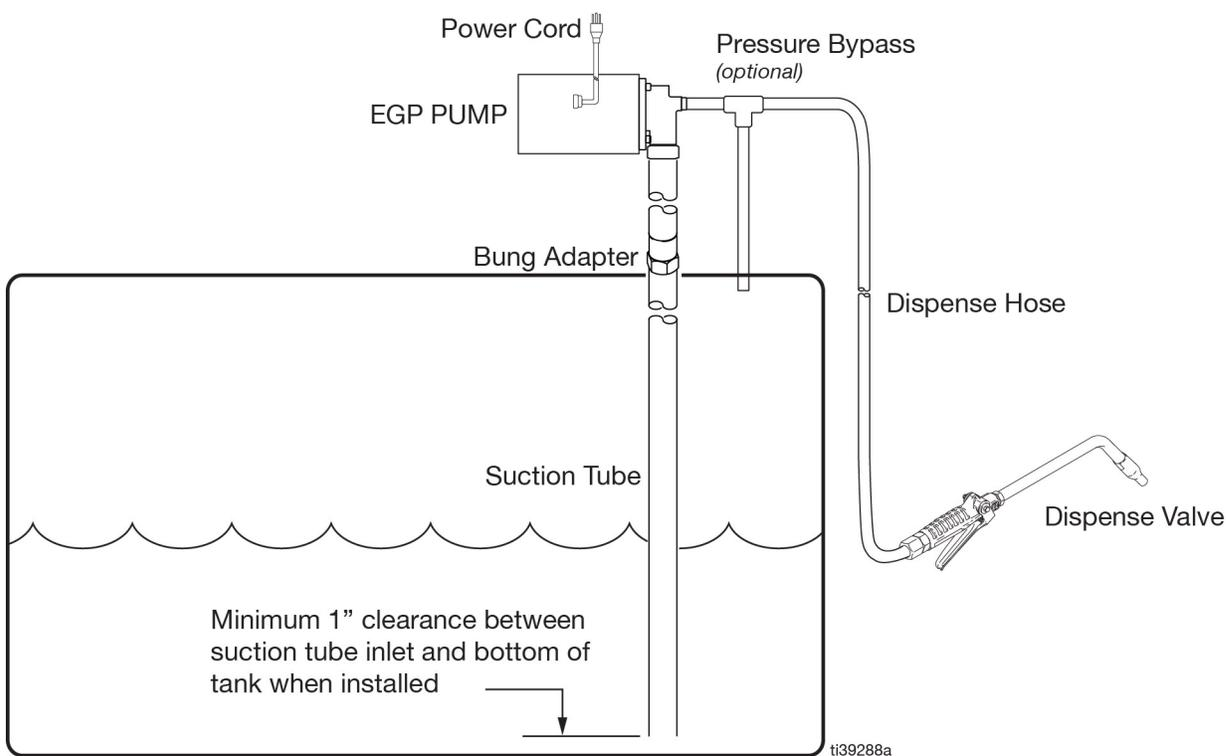
**FIG. 1: Typical Installation - Option 1: Pump and Dispense Valve**
