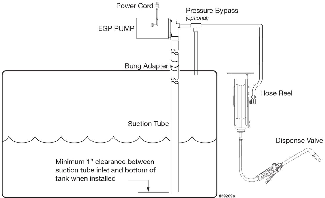
**FIG. 2: Typical Installation - Option 2: Pump with Hose Reel**
