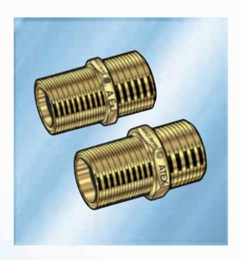
**AM-D Series** Male x Male Adaptors provide a method of matching female threadforms of the same size or of dissimilar size and threadform, while maintaining Ex certification. Ex Male x Male Adaptors are not certified for connecting Exd Enclosures.
