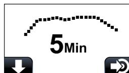
To change the interval of barometric recording points, **press** your **SET** key and choose 5, 10, 30 or 60 minutes. The default setting for recording the barometer curve is 5 minutes.
