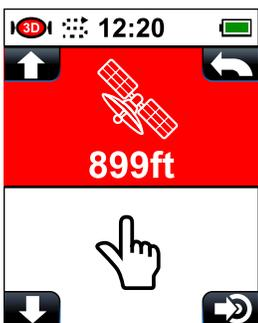
2. **Manually set altitude:** To manually set the altitude benchmark, **press** the **CHANGE SETTING** key once to highlight the Manual setting (finger) icon. **Press** the **POWER** key to open the manual setting window. Using your **SCROLL** key or the **CHANGE SETTINGS** keys, enter the height you would like for your benchmark.
