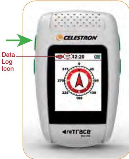
Your trail data is now being recorded. To turn off the trail data recording function, *press* and *hold* the **SCROLL** key until the Data Log icon goes away.
