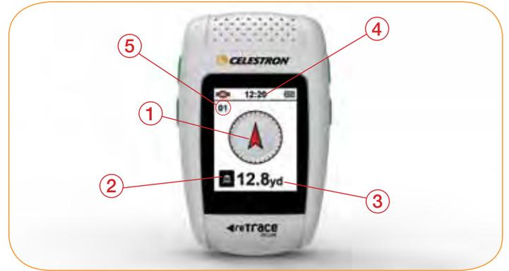
1. 32 Way Arrow – The 32 Way Arrow points in the direction of your saved Waypoint or POI. If the GPS signal is not fixed, the display will be empty. If the current window has no POI assigned, the arrow will be gray.
