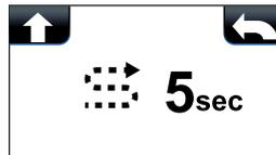
The Data Log setting tells the reTrace™ Deluxe how often to record data. This is a powerful tool that collects info about your travels that can be saved and uploaded to the reTrace™ Deluxe software for analyzing. The default time for the Data Log Period is 5 seconds. **Press** your **SET** key to select and make changes. This window appears:
