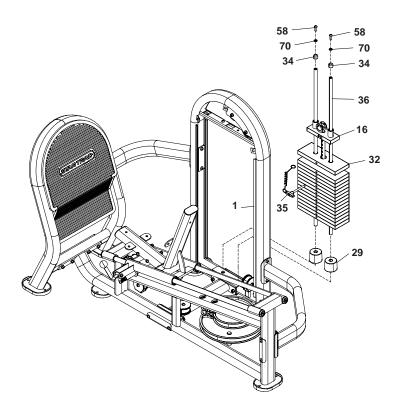
Install one rubber cap (34) onto each weight stack guide post (36).
