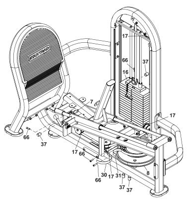
Insert one end of the weight belt (31) through the slot in the top plate belt clamp until approximately one inch of the free end of the belt protrudes from the slot in the opposite side of the clamp.
