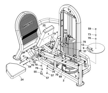
Secure the flywheel cover (13) to the range-of-motion flywheel (8) using one screw (59), spring washer (73) and washer (70). Tighten the screw securely.
