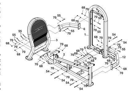
Secure the main frame to the lower crossbeam using two screws (54), four washers (70), and two lock nuts (68). Tighten the nuts securely.
