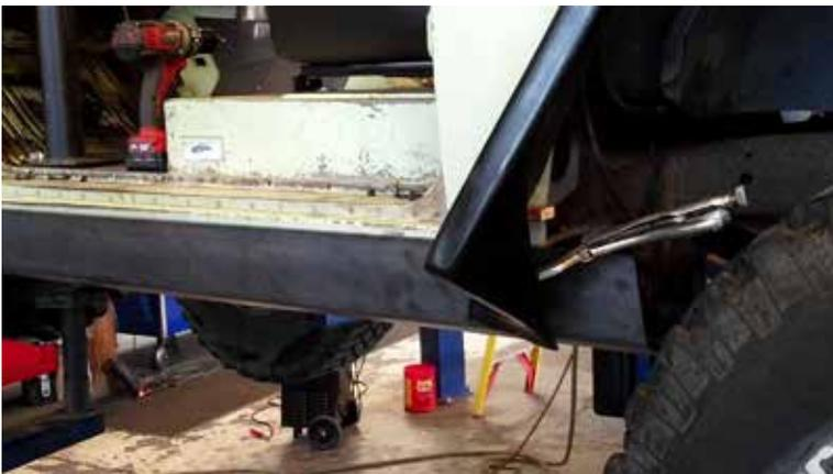
Holding Rail in place while working. You can use a floor jack, c-clamp or vise grip type clamp.
