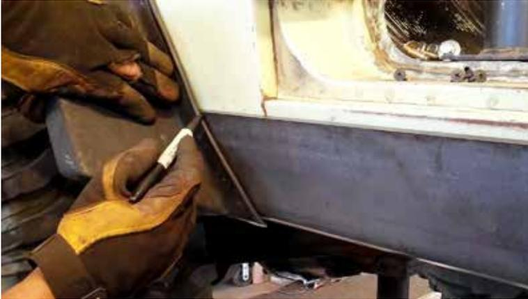
Marking Rail for trimming to fit flare. Make sure front and rear of Rail are parallel with the door opening and not leaning to the front or rear.
