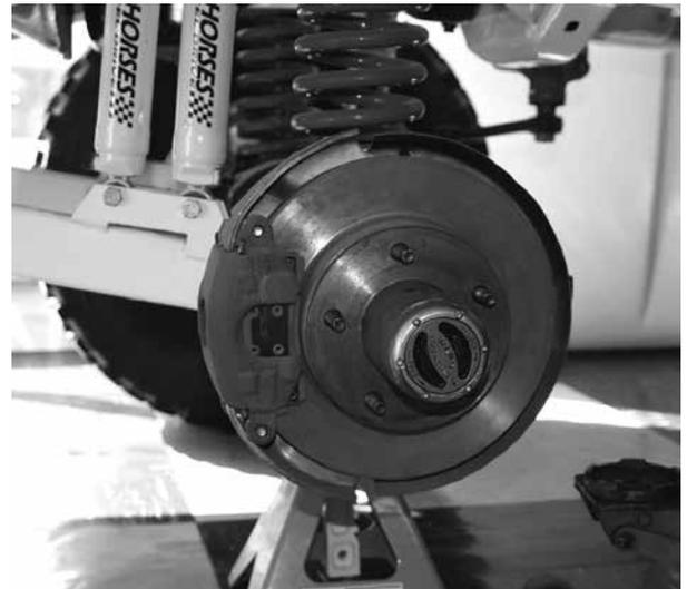
Be sure to mount calipers with the bleed screws up. The brake hoses should be mounted up and then into the bracket on the front end. DO NOT mount the hose back and into the bracket because it could rub on the tire or wheel. Double check hose install by turning wheels full right and full left while watching the hose. Make sure there is no interference anywhere.
