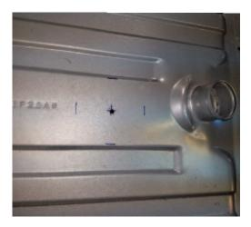
7 Then cut a 4 ½" hole using a 4 ½" hole saw with a slow speed drill.
