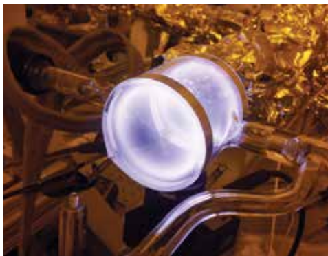
James Maxwell's helium-3 polarization experiment in his lab at MIT.
