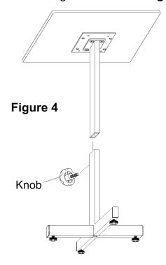
**Height Adjustment:** To adjust the height of the unit hold the inner tube with one hand and loosen the knob with the other hand. Set height at desired level and tighten knob.
