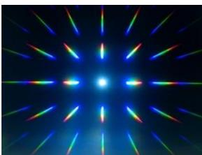
These highly efficient, double axis, holographic diffraction grating lenses separate light from any source into its spectral components for study and analysis. Lenses are mounted in sturdy cardboard frames. Sold in sets of 10.
