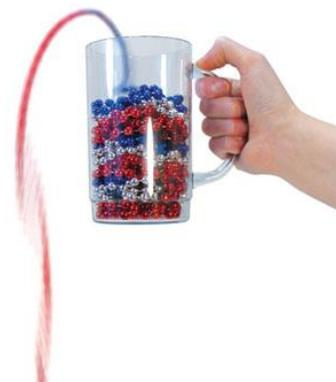
The Polymer Bead Demonstration allows one to model the tubeless siphon phenomena.
