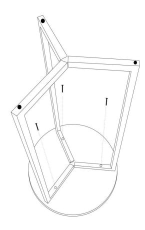
Step 2Screwing the leg ( A) in to the table top (B)
