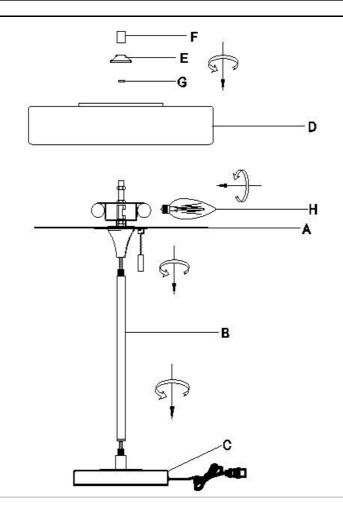
Step: Remove all accessories from the outer box. First install the straight tube (B) onto the lamp holder (A) accessory and then lock it onto the base (C). Install the bulb (H) onto the lamp holder (A) first, and then install the lampshade (D) and lock it with nuts (G). Finally, install the decorative element (E) and lock it with decorative particles (F). After installing all the accessories, manually adjust the lampshade (D) to balance it.
