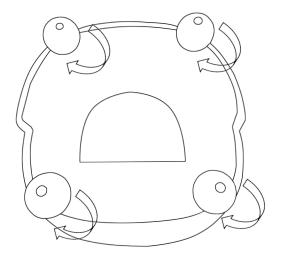
Turn the chair upright and you can adjust legs by adding plastic washers(HW1) before rotating to make sure it is level.
