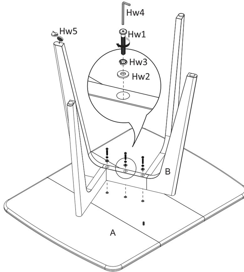
STEP 1: Assemble Legs (B) into Table Top (A) by using Bolts (Hw1), Flat Washer (Hw2), Split Lock Washer (Hw3). Fully tighten by Allen key. Attach Felt pads (Hw5) on the bottom.
