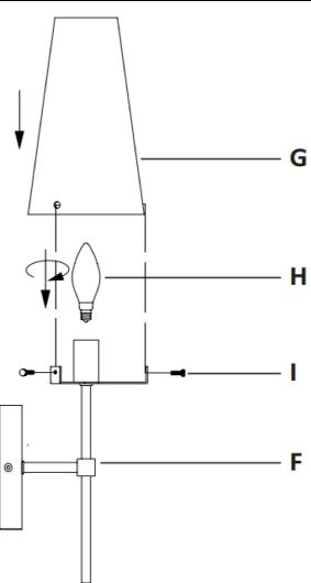
**Step 5:** Insert the Bulbs(H) into the sockets of the Fixture Body (F) until secure. Unscrew the three Thrumbscrews (I) from the Fixture Body (F), place the Glass shade (G) over the socket. Align the three holes of the Glass Shade (G) and the Fixture Body (F), then secure with the Thrumbscrews (I).
