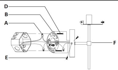
**Step 4:** Place the canopy of the Fixture Body (F) over the outlet box, align the two holes of the mounting bracket (B) and the canopy of the Fixture Body (F), then tighten the Support Screws (E).
