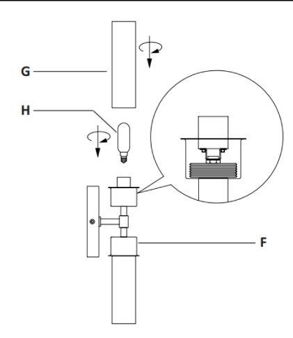
**Step 5:** Insert the Bulbs (H) into the sockets of the Fixture Body (F) until secure. Insert the inner threaded end of the Glass Tube (G) into the socket cap of the Fixture Body (F), then tighten the Glass Tube (G).
