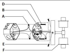
**Step 4:** Place the canopy of the Fixture Body (F) over the outlet box, align the two holes of the mounting bracket (B) and the canopy of the Fixture Body (F), then tighten the Support Screws (E).
