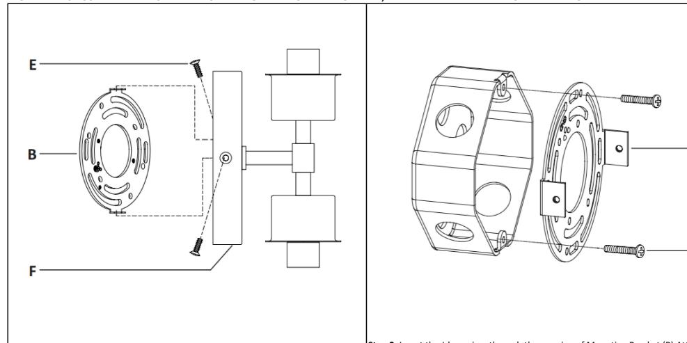
**Step 1:** Unpack all parts from carton carefully. Unscrew the two Support Screws (E) from the Mounting Bracket (B). Remove the Mounting Bracket (B) from the Fixture body (F), and keep the Support Screws (E) for later use.
