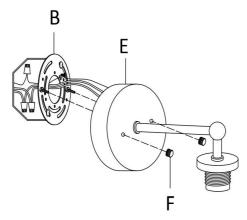
**Step 3:** Tuck wires inside junction box. Attach the Lamp Body (E) to the Mounting Plate (B) and secure with Screwed Ball (F).
