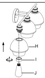
Step 4:Place the glass shade (H) on the socket and tighten it clockwise with the socket ring (I) Insert the bulb (J) into the socket
