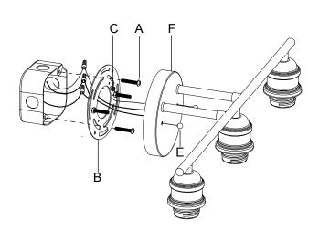
Step 3: Attach the lamp body (F) to the Mounting plate (B) and secure with Round nut (E)
