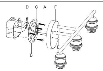
Step 1: Secure mounting plate (B) to outlet box with mounting screws (A).
