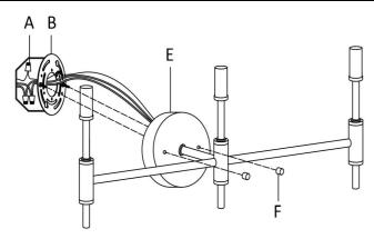
Step 3: Tuck wires inside junction box. Attach the Lamp Body (E) to the Mounting Plate (B) and secure with Screwed Ball (F).
