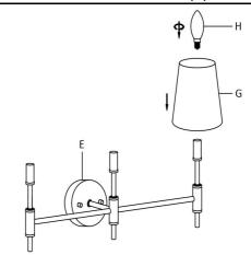
Step 4: Insert the Shade (G) to the socket of the Lamp Body (E). Insert the Bulb (H) into the Socket.
