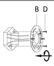
Step 1: Unpack all parts from cartons carefully. Separate the Mounting Plate (B) from the Lamp Body (E) by removing the Screwed Ball (F) anti-clockwise. Fix the Mounting Plate(B) to the junction box with Mounting Screw (D).
