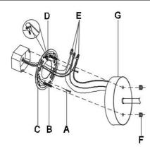
**Step 3:** Attach the Canopy (G) to the Mounting Plate (C), and tix it by turning the canopy nut (F).
