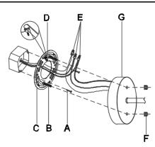
**Step 3:** Attach the Canopy (G) to the Mounting Plate (C), and tix it by turning the canopy nut (F).
