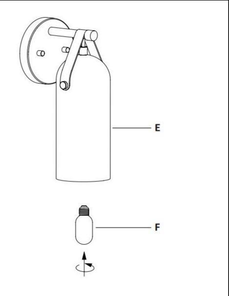
Step 5: Insert the Bulbs (F) into the sockets of the Fixture Body (E) until secure.
