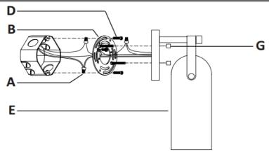
**Step 4:** Place the Fixture Body (E) over the outlet box, and ensure the heads of the support screws of the Mounting Bracket (B) come through the holes of back of the Fixture Body (E). Tighten the Canopy Nuts (G) onto the protruding support screwsof the Mounting Bracket (B) until the Fixture Body (E) is held firmly against the wall.
