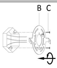
**Step 1:** Unpack all parts from cartons carefully. Separate the Mounting Plate (B) from the Lamp Body (F) by removing the Retaining Screw (E) counter-clockwise. Attach the Mounting Plate(B) to the junction box with Mounting Screw (C).
