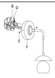
**Step 3:** Tuck wires inside junction box. Attach the Lamp Body (F) to the Mounting Plate (B) and secure with Retaining Screw (E).
