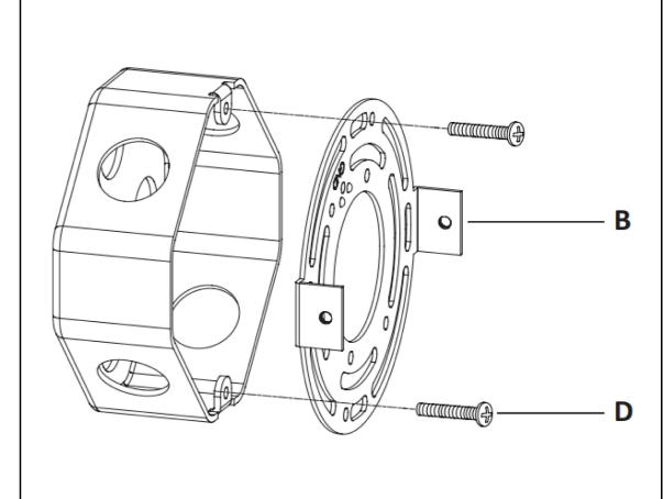
**Step 2:** Insert the J-box wires through the opening of Mounting Bracket (B). Attach the Mounting Bracket (B) onto the J-box and secure it by turning the 2 Mounting Screws (D) clockwise until tight.
