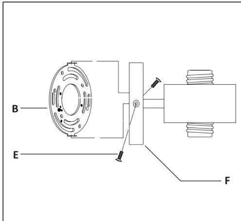
**Step 1:** Unpack all parts from carton carefully. Unscrew the two Support screws (E) from the Mounting Bracket (B). Remove the Mounting Bracket (B) from the Fixture body (F), and keep the Support Screws (E) for later use.
