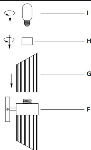
**Step 5:** Unscrew the Socket Rings (H) from the socket of the Fixture Body (F), place the Glass Shade (G) over the socket and secure with the Socket Ring (H). Insert the Bulbs (I) into the sockets of the Fixture Body (F) until secure.
