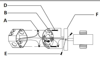
**Step 4:** Place the canopy of the Fixture Body (F) over the outlet box, align the two holes of the mounting bracket (B) and the canopy of the Fixture Body (F), then tighten the Support Screws (E).
