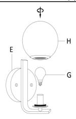
**Step 4:** Insert the Bulb (G) into the Socket. Attach the Glass Shades(H) onto the socket cap of the Lamp Body (E).
