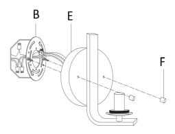
**Step 3:** Tuck wires inside junction box. Attach the Lamp Body (E) to the Mounting Plate (B) and secure with Retaining Screw (F).
