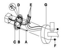
Step 3:Install the Mounting Plate(C) to the junction box with Machine Screw(A),Attach the Canopy(G) to the Mounting Plate(C),and tix it by turning the canopy nut(F)
