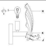
Step 3:Use the decorative ball screw(J) to thread through the plastic gasket(K) to rotate and fix the glass(H) to the position of the lamp body screw, and then fix the bulb(I) into the lamp heolder
