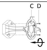
Step 1: Unpack all parts from cartons carefully. Separate the Mounting Plate (C) from the Lamp Body (G) by removing the Retaining Screw (F) anti-clockwise. Fix the Mounting Plate(C) to the junction box with Mounting Screw (D). If the cord of the Lamp Body (G) is too long, the cut the excess cord. Make sure to leave at least 6-in for wiring. Pull the power cord into the face plate of the lamp Body (G) and separate it, Tail peeling 1/2".
