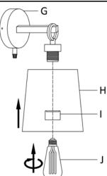
Step 3: Tuck wires inside junction box. Attach the Lamp Body (G) to the Mounting Step 4: Place the Shade (H) over the socket, the secure with the Socket Ring (I). Insert the bulbs (J) into the Socket.
