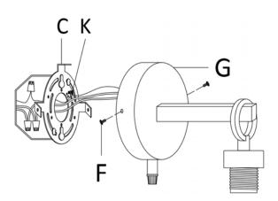
Plate (C) and secure with Retaining Screw (F).
