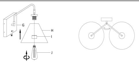
**Step 4:** Place the Shade (H) over the socket, then secure with the Socket Ring (I). Insert the bulb (J) into the Socket. Hold the arm of the Lamp Body (G) can turn the lamp body left and right, can adjust the direction of shade (H).
