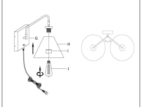
**Step 2:** Place the Shade (H) over the socket, then secure with the Socket Ring (I). Insert the bulb (J) into the Socket. Hold the arm of the Lamp Body (G) can turn the lamp body left and right, can adjust the direction of shade (H).
