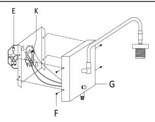
**Step 3:** Tuck wires inside junction box. Attach the Lamp Body (G) to the Mounting Plate (C) and secure with Retaining Screw (F).
