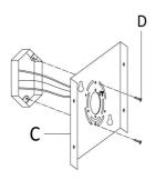
**Step 1:** Unpack all parts from cartons carefully. Separate the Mounting Plate (C) from the Lamp Body (G) by removing the Retaining Screw (F) anti-clockwise. Fix the Mounting Plate(C) to the junction box with Mounting Screw (D). If the cord of the Lamp Body (G) is too long, the cut the excess cord. Make sure to leave at least 6-in for wiring. Pull the power cord into the face plate of the lamp Body (G) and separate it, Tail peeling 1/2".
