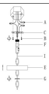
Step 4: Install the Mounting Plate(C) to the junction box with Mounting Screw (B).
