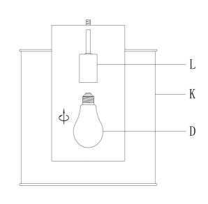
Step 6: Insert the bulb (D) into the Socket (L).
