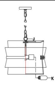
Step 4: Insert the bulb (K) into the socket of the shade (J),
