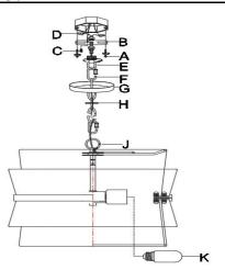
Step 2:Lock the screw collar nut (E) onto the mounting plate (B). Use a chain (F) to pass through the canopy (G) and lock it with a threaded collar (H). Hang the upper end of the chain (F) on the screw collar nut (E) and the lower end on the lifting ring of the shade (J).
