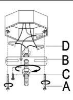
Step 1: Secure mounting plate (B) to outlet box with mountings crews (A).
