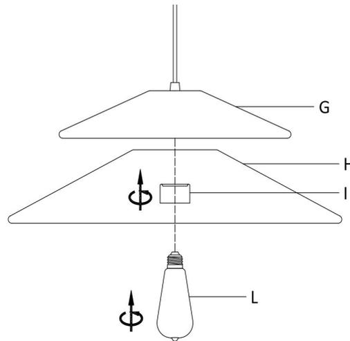
**Step 5: Put the Shade(H) on socket of the Lamp Body (G), then fasten it by Socket Ring(I). Insert the Bulb (L) into the Socket.**
