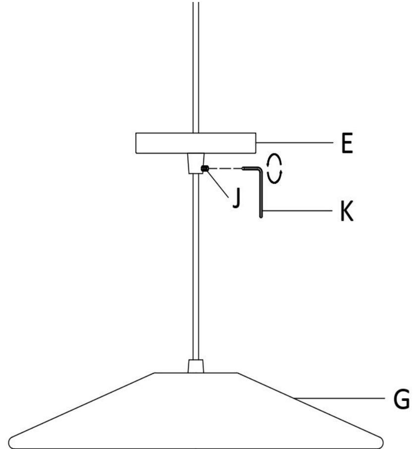
**Step 2:** Loosen the Screw (J) with a Spanner (K), adjust the length of the wire, and alter the cord to the desired length, Tighten the Screw (J) to secure.
