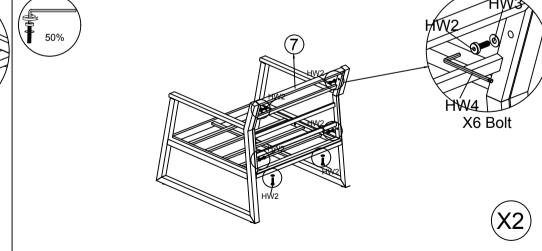
STEP 4: Connect Seat Chair Frame (6) & Right Frame (5), Left Frame (4), tighten Bolt (HW2), Flat Washer (HW3) with Allen Key (HW4).
