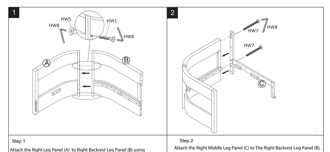
Using Screws (HW7) and the Allen key (HW8) as shown above.
