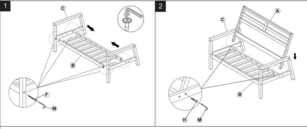
Step 1  $\begin{tabular}{ll} Attach Frame Leg (C) to Frame Seat (B) ,use Screw (F) tighten with allen key (M). \end{tabular}$
