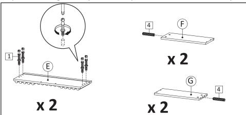
**STEP1**: Insert Cambolt (HW1) into Front Drawer (E). Insert Dowel Small (HW4) into Side Drawers (F & G).
