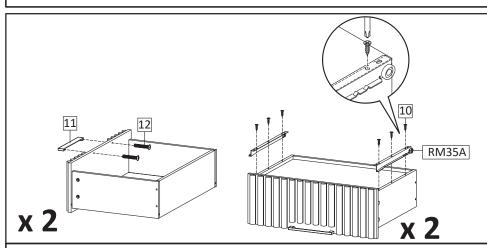
**STEP3**: Use Screw M4x22mm (HW12) to attach Handle (HW11) to the Front Drawer.
