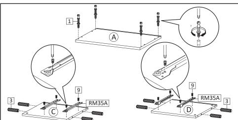
**STEP5**: Insert Cambolt (HW1) into Top Board (A),and Insert Dowel Big (HW3) into Side Board Left (C) and Side Board Right (D). Continue with securing part of the Drawer Runner (HW RM35A) into position as the above image, using screw M6x10.5mm (HW9).
