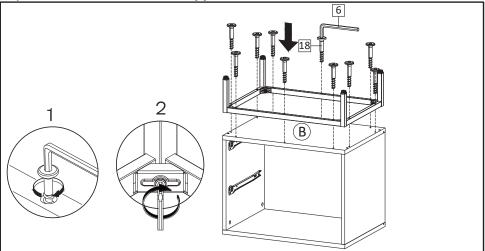
**STEP10**: Install the assembled leg unit from Step 9 onto the Bottom Board (B). Then, insert the M6.4 x 35 mm screws (HW18) into all the Corner Braces (HW13), Support Metal Leg 1 (HW15), and Support Metal Leg 2 (HW16). Tightenall screws using the Allen Key (HW6).
