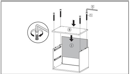
**STEP7**: Attach Back Board (J) and Insert Bottom Board (B), secure with Screw M7x50mm (HW5), tighten screws using Allen Key (HW6).
