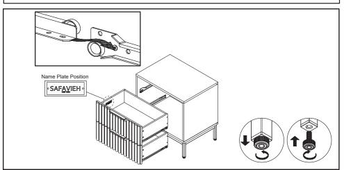
**STEP12**: Hold the sides of the drawer and position the rail wheels, one the back of drawer and the others on the side boards according to the image. Slide the drawer on by one into the nightstand. Place your f urniture on a level floor. The legs come with adjustable levelers, adjust them as needed until the furniture sits steadily on the floor.
