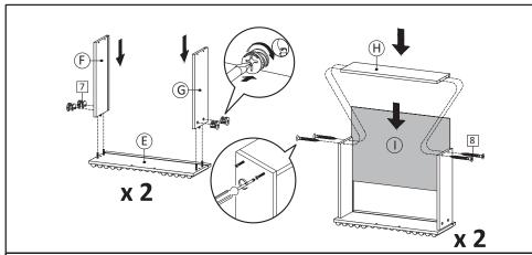
**STEP2**: Combine Side Drawers (F & G) into Front Drawer (E) then tighten camlock (HW7) using screwdriver.Insert Bottom Drawer (I) with laminated face facing upward then put Back Drawer (H) and secure with Screw M8x39mm (HW8).
