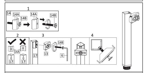
**STEP8**: First, remove the M6 x 35 mm screw (HW14B) from the Support Corner Brace (HW14A). Second, insert the Support Corner Brace (HW14A) into the Leg (HW17), ensuring that the hole in the Support Corner Brace aligns with the hole in the Leg. Third, insert the M6 x 35 mm screw (HW14B) into the hole in the Corner Brace (HW13), and insert it into the hole in the Leg, then tighten it slightly.
