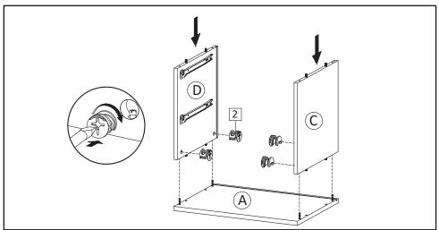
**STEP6**: Attach Side Board Left (C) and Side Board Right (D) into Top Board (A). Secure with Camlock Big (HW2) and tighten it using screwdriver.
