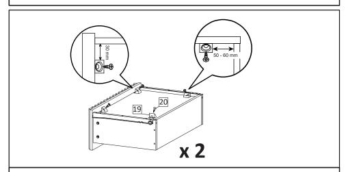
**STEP4**: Insert the Screw M3.5x15.5mm (HW20) and wedge (HW19) into the bottom of the drawer according to the picture.
