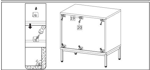
**STEP11**: Use Wedge (HW19), Screw M 3.5 x15.5 (HW20) to tighten the back of night stand by using screwdriver. Please align the top board and bottom board in  $90^{\circ}$  position againt the side board, before securing the wedges (HW19)
