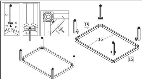
**STEP9**:Place Support Metal Leg 1 (HW15) and Support Metal Leg 2 (HW16) on the floor as shown in the image. Then, install the prepared leg (HW17). Ensure that the Corner Brace (HW13) hooks into the holes of Support Metal Leg 1 (HW15) and Support Metal Leg 2 (HW16). Use the Allen Key (HW6) to slightly tighten the screws, just enough to hold the Support Metal Legs in place. Do not fully tighten them. Repeat this process for the remaining legs.
