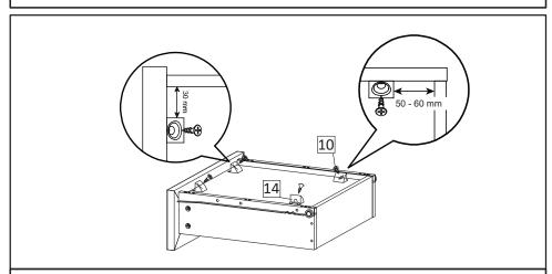
**STEP4**: Insert the Screw M3.5x15.5mm (HW10) and wedge (HW14) into the bottom of the drawer according to the picture.
