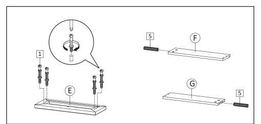
**STEP1**: Insert Cambolt (HW1) into Front Drawer (E). Insert Dowel Small (HW5) into Side Drawers (F & G)
