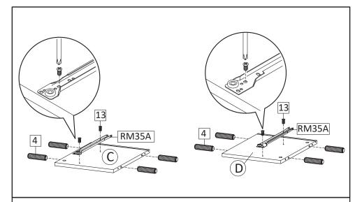
**STEP6**: Insert Dowel Big (HW4) into Side Board Left (C) and Side Board Right (D). Continue with securing part of the metal runner (HW RM35A) into position as the above image, using screw M6x10.5mm (HW13).
