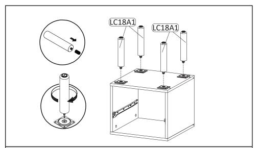
**STEP10**: Insert Leg (LC18A1) into Mounting Plate, tighten by rotating . the leg clockwise.
