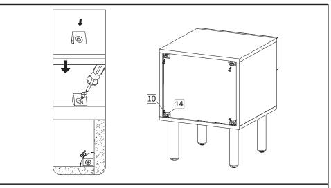
**STEP12**: Use Wedge (HW14), Screw M 3.5 x15.5 (HW10) to tighten the back of Night Stand by using screwdriver. Please align the top board and bottom board in  $90^{\circ}$  position against the side board, before securing the wedges (HW14).
