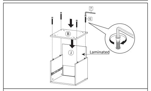
**STEP8**: Insert Back Board (J) with laminated facing front side followed by Bottom Board (B), secure with Screw M7x50mm (HW6), tighten screws using Allen Key (HW7).
