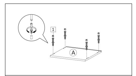
STEP5: Insert Cambolt (HW1) into Top Board (A).
