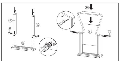
STEP2: Combine Side Drawers (F & G) into Front Drawer (E) then tighten camlock small (HW3) using screwdriver.
