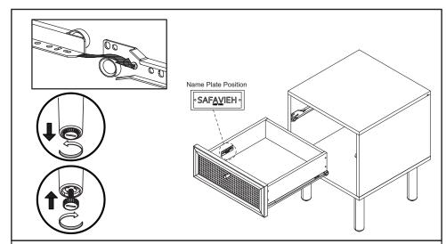
**STEP11**: Hold the sides of drawer, position the wheel of rail at drawer back and the wheel of rail at side boards, according to the image. Slide in the drawer into the night stand.
