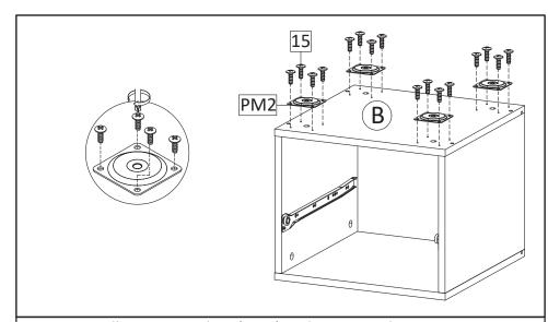
**STEP9**: Install Mounting Plate (PM2) and secure with screw M4.5x12.5mm (HW15) on Bottom Board.
