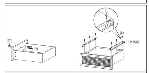
**STEP3**: Use Screw M4x22mm (HW9) to attach Handle (HW8) to the Front Drawer.
